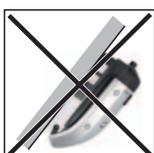
Do not install the inverter such that it overhangs.
