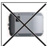
Do not install the inverter horizontally on a vertical wall or pillar.
