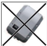
Do not install the inverter at an angle on a vertical wall or pillar.
