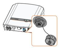
5. Align the communication connector and the **Meter** terminal. Plug the connector and make them engage perfectly until a "Click" is heard or felt. Secure the screw nut to the inverter bottom.
